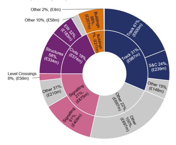
3.11 As indicated by the inner ring, expenditure on Track, Signalling, Civils and Buildings accounted for 78% of the total. Asset classes are further split into subasset class or work type in the outer ring of the figure. For instance, the Track and Switches & Crossings sub-asset classes accounted for 85% of average total Track renewals expenditure.
