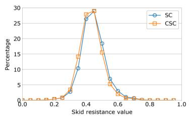
Figure B-1 The distributions of SC and CSC values for a sub-set of the NH network
