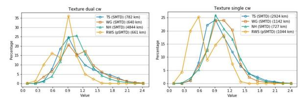
Figure 4-7 Histograms of texture depth values for dual carriageways (left) and single carriageways (right)
