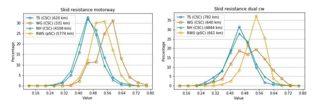
Figure 4-9 Histograms of skid resistance values for motorways (left) and dual carriageways (right)
