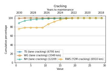
Figure 4-5 Cumulative frequency distribution for cracking values
