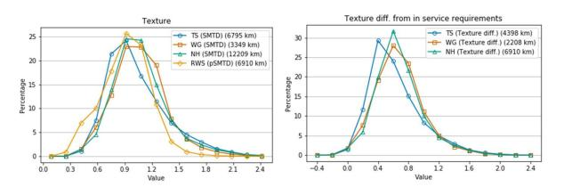
Figure 4-6 Histogram of texture depth values, and differences from in service requirements
