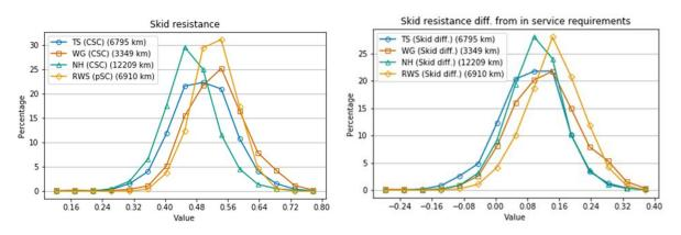
Figure 4-8 Histogram of skid resistance values and difference from in-service requirements
