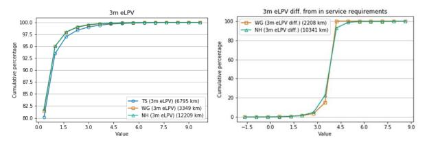
Figure 4-1 Cumulative frequency distribution of 3m eLPV values, and distribution of 3m eLPV difference from in-service requirements
