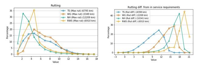
Figure 4-3 Histogram of rutting values, and differences from in service requirements
