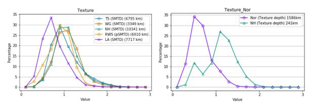
Figure 6-1 Whole network results for the local authority comparison for texture depth (left) and comparing Norfolk and NH (right)
