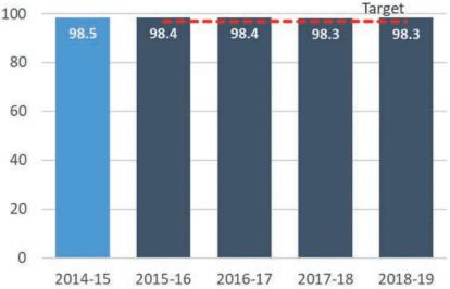
Network availability is a measure of the length of road lanes that are open to traffic as a percentage of the total length of road lanes on the network. Performance is calculated over a rolling year. At the end of 2018-19, network availability on the strategic road network was 98.3%, which is the same as the previous year, and above the target of 97%.
