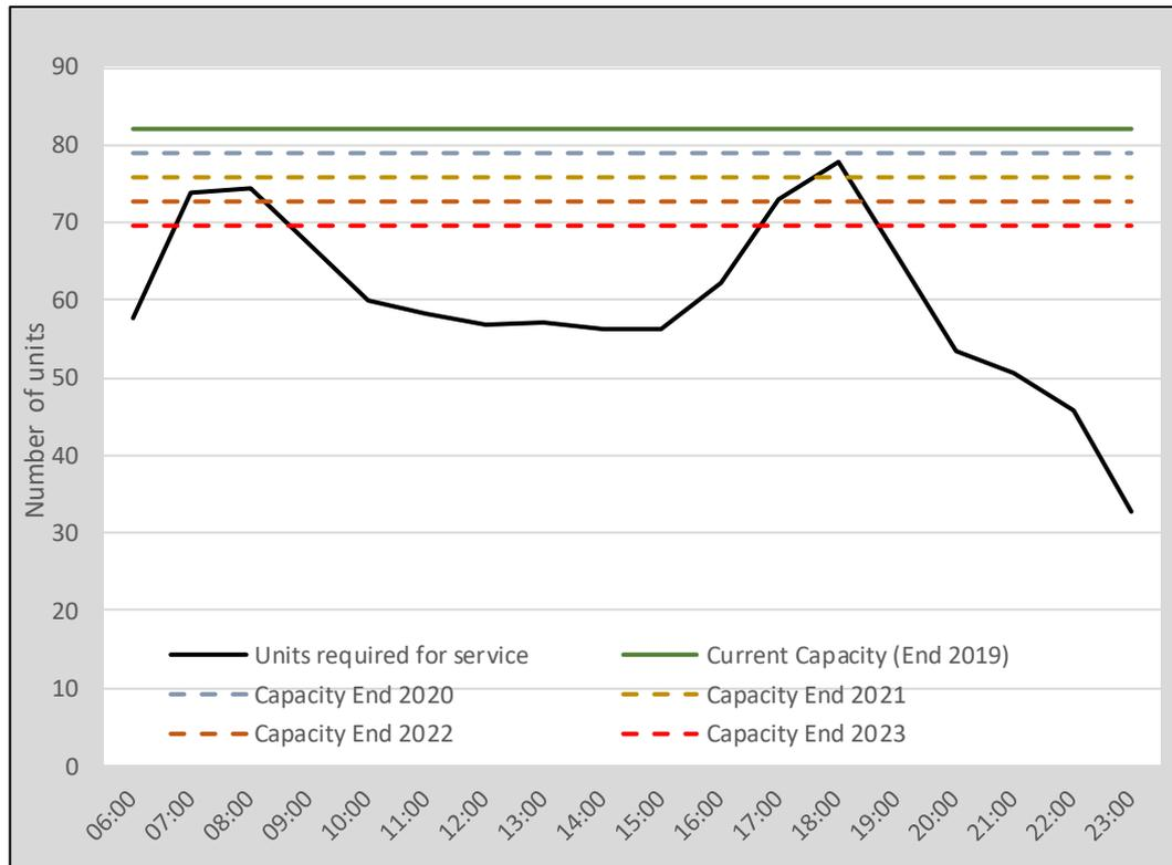
**Figure 5 Units required and units available at 10% ATP degradation per year**
