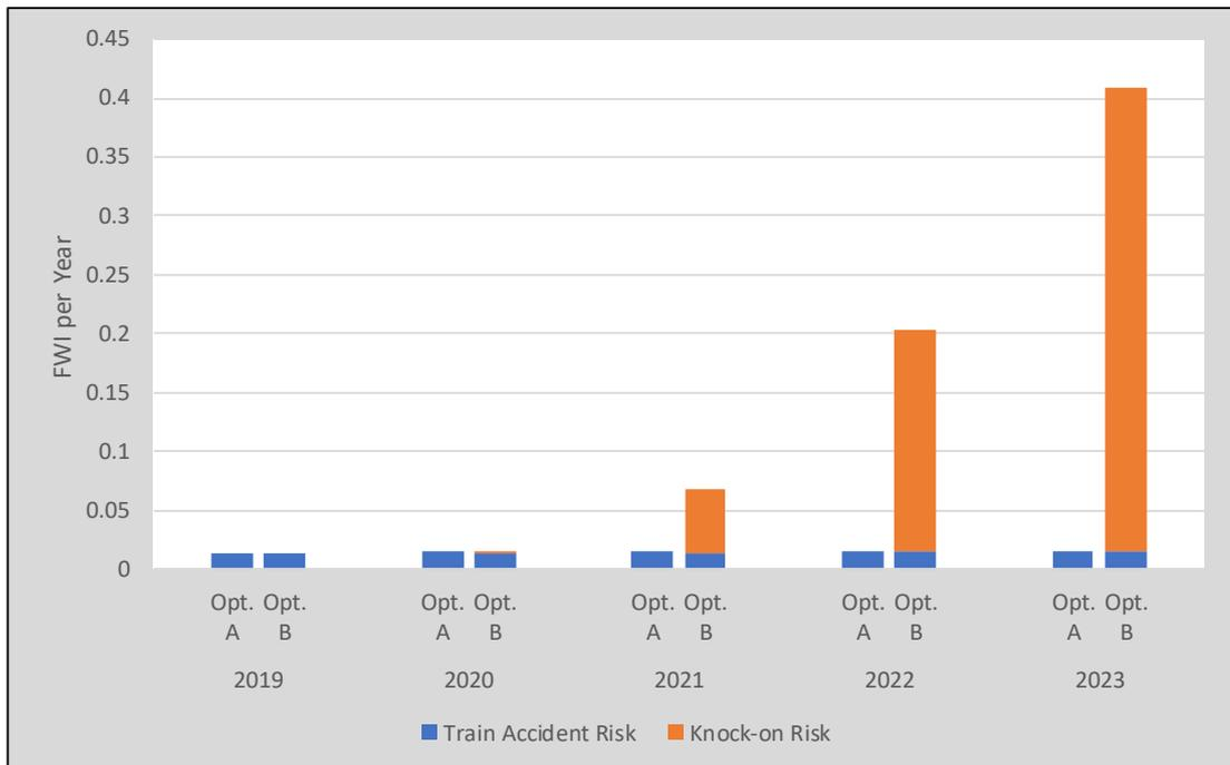
**Figure 10 Comparison of the risk for Option A and Option B at 30% degradation**
