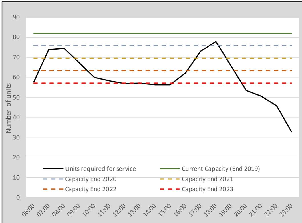
**Figure 6 Units required and units available at 30% ATP degradation per year**
