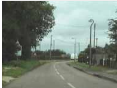
Figure 25 26: the level crossing sign, positioned on the left-hand side is obscured from the vehicle driver's view.
