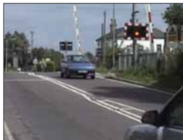
Figure 22 48: drivers have been observed ignoring the amber light, although they have had sufficient time to stop at the lights. The vehicle driver approaching the crossing continues to drive straight over.
