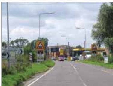
Figure 21 15: the approach to Tallington is cluttered with yellow advertising signs and a yellow branded petrol station. These all make it very difficult for approaching vehicle drivers to identify the similar coloured crossing signage.
