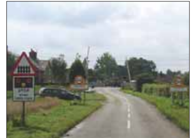
Figure 26 88: the 30mph zone is positioned close to the crossing, after a 60mph zone on a long straight road.
