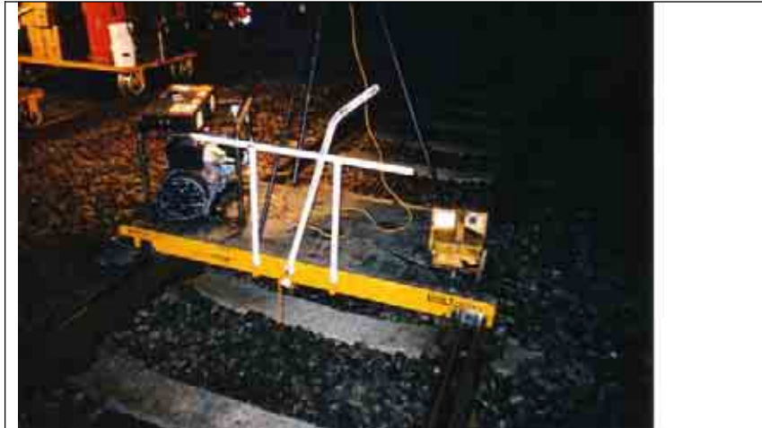
Figure 45. Rail trolley showing a slot-in handle for pushing, and a brake lever at an appropriate height.
