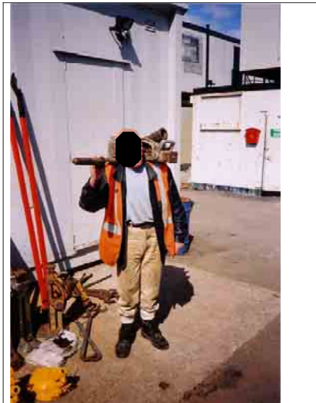
Figure 43. The usual method for carrying a Duff Norton rail jack and handle.
