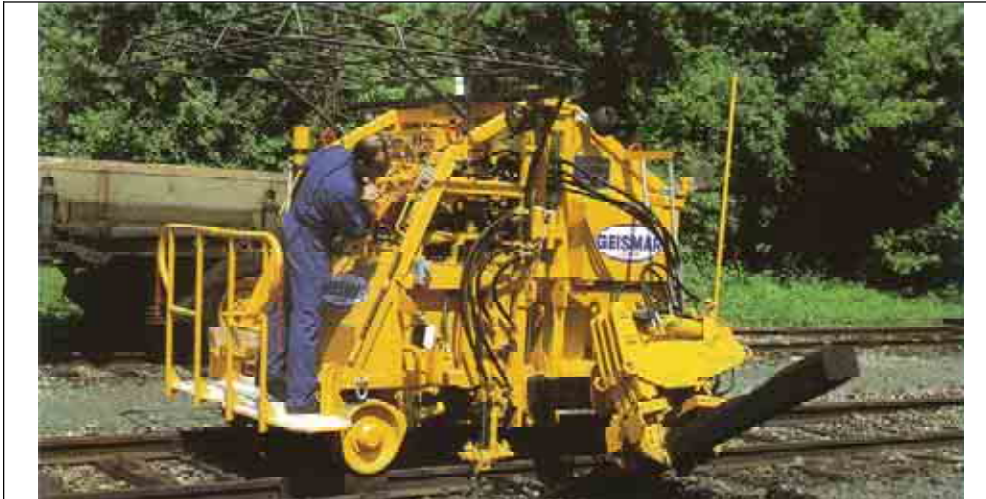
Figure 27. An example of a mechanical sleeper replacement machine. (Source: Geismar catalogue)
