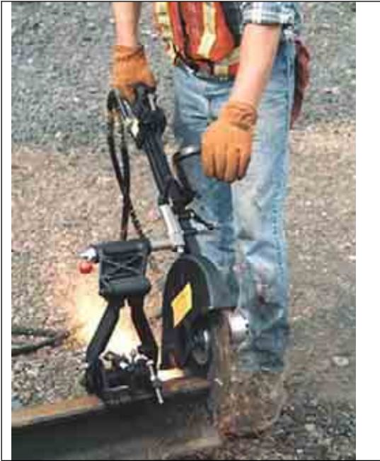
Figure 38. A long handled disc cutter (Source: Stanley Tools)
