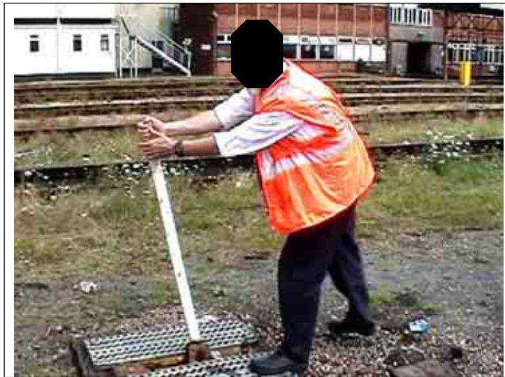
Figure 13. Points lever operation - start of pull.
