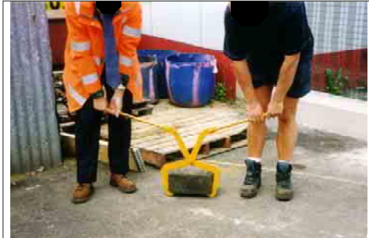
Figure 41. Demonstration of the wooden sleeper tongs.
