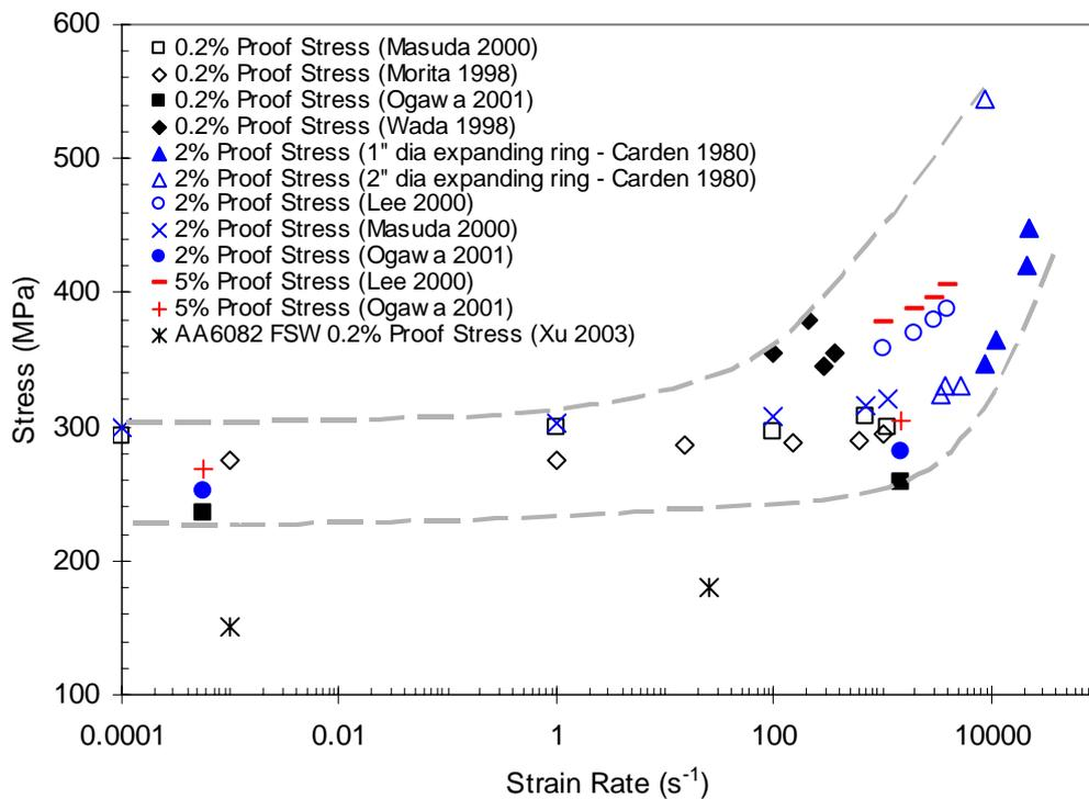
Figure 2: Flow stress properties of AA6061-T6 obtained by several authors as a function of strain rate. Also shown are the properties obtained by Xu and Gittos (2003) for alloy AA6082 after friction stir welding, showing an increased strain rate effect compared to the T6 treated alloys.
