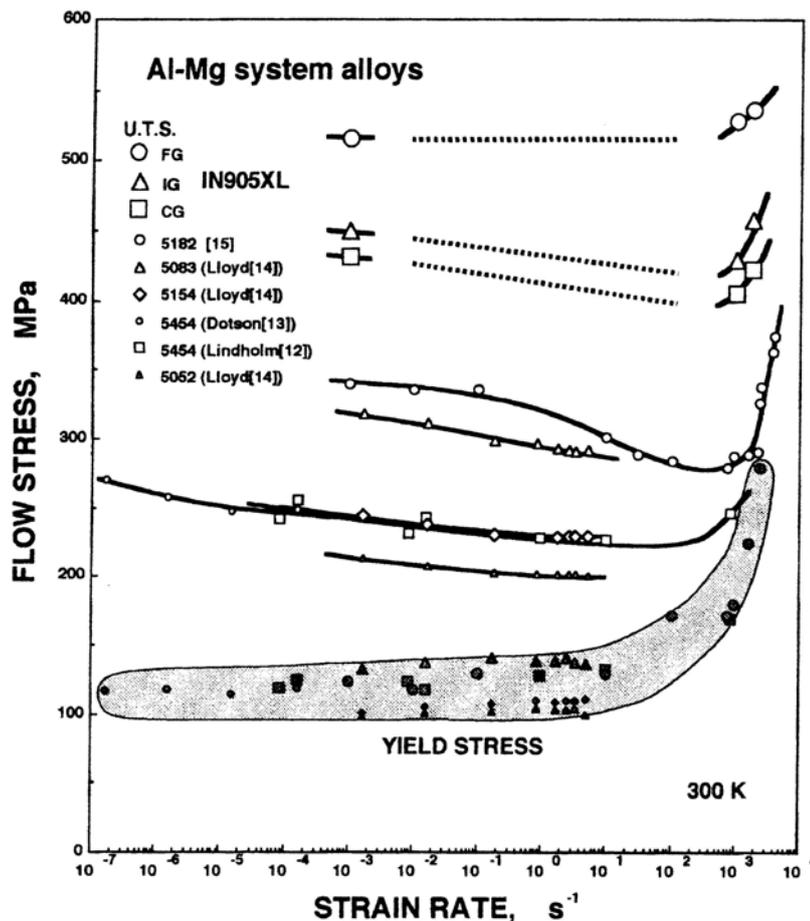
Figure 1: Summary of strain rate dependence of mechanical properties of AA5xxx series Al-Mg alloys. From Mukai *et al* (1995)
