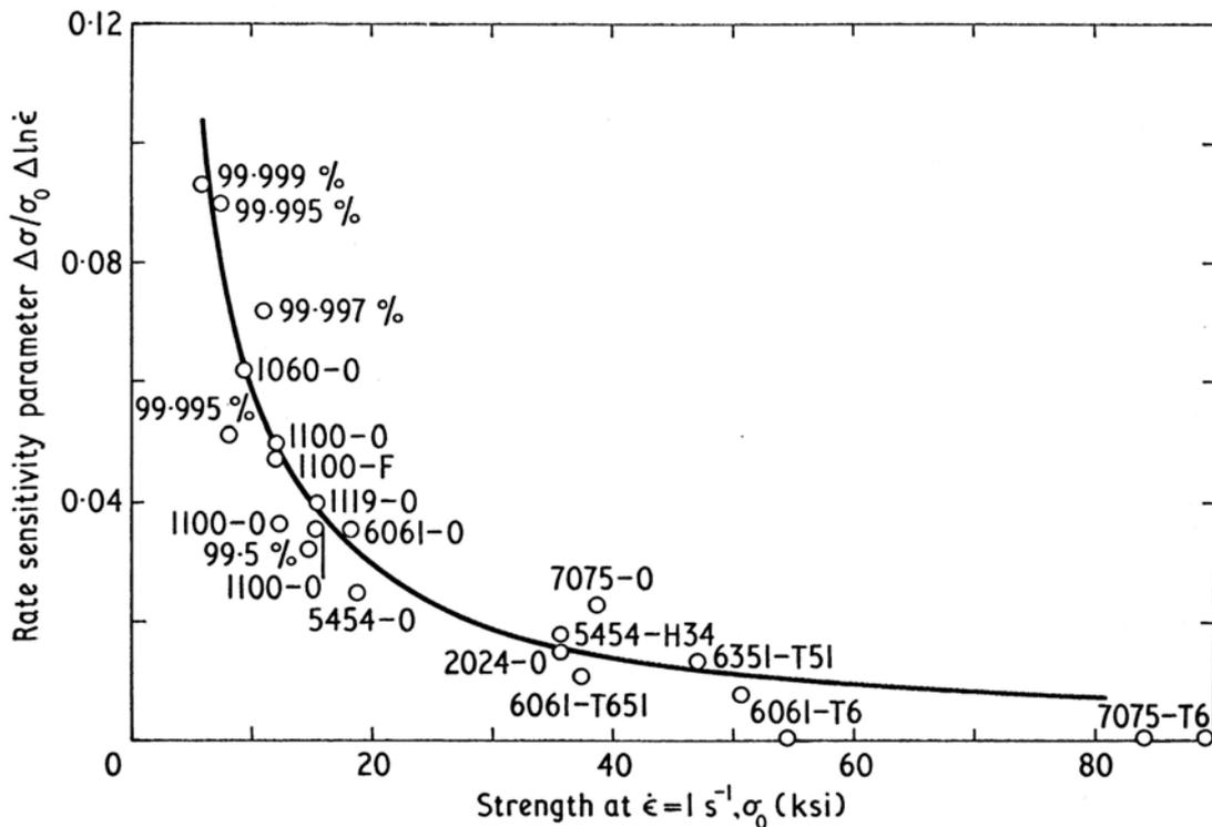
Figure 3: Variation in rate sensitivity parameter as a function of alloy strength. From Lindholm (1974).
