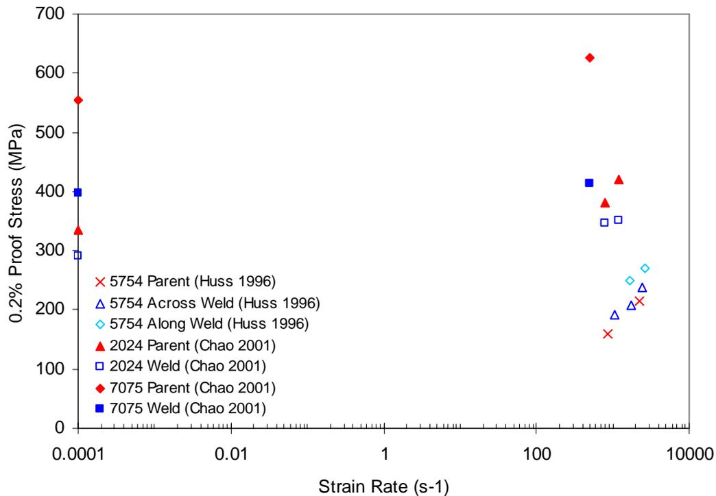
Figure 4: 0.2% Proof stress data for aluminium alloy welds and parent materials as a function of strain rate.
