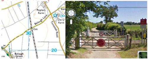
It is normally protected by gates, or lifting barriers (when authorised by ORR), on both sides of the railway. The gates, normally closed across the road and hung so as to open away from the railway, are operated by the road users. Barriers are normally closed across the road. A sign describing correct crossing procedure, including the use of any telephones, is displayed to road users on each side of the crossing.
