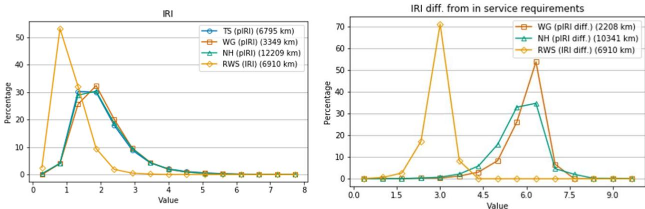
Figure 4-2 Histogram of IRI values, and difference from in-service requirements<sup>9</sup>
