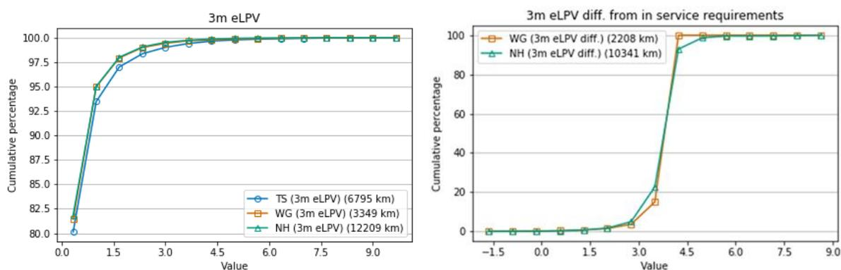
**Figure 4-1 Cumulative frequency distribution of 3m eLPV values, and distribution of 3m eLPV difference from in-service requirements**
