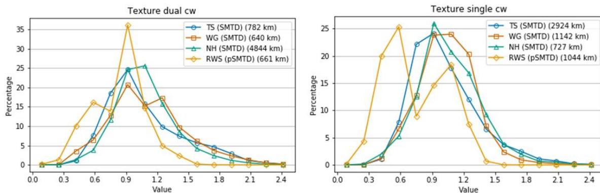
**Figure 4-7 Histograms of texture depth values for dual carriageways (left) and single carriageways (right)**
