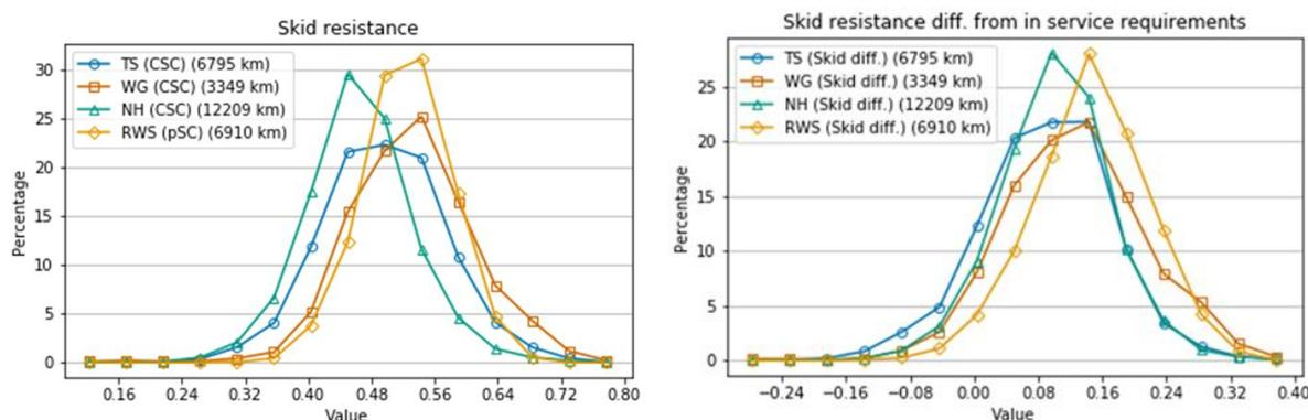
**Figure 4-8 Histogram of skid resistance values and difference from in-service requirements**
