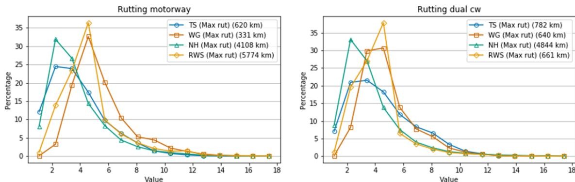
**Figure 4-4 Histograms of rutting values for motorways (left) and dual carriageways (right)**
