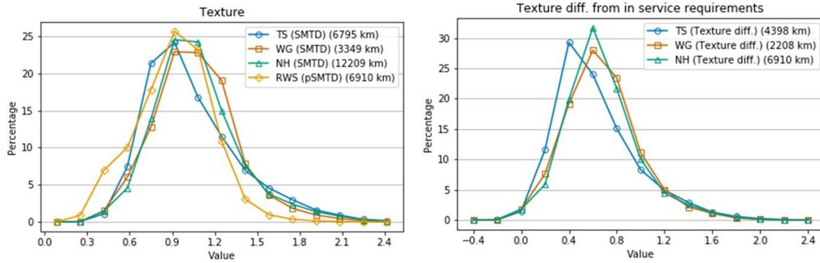
**Figure 4-6 Histogram of texture depth values, and differences from in service requirements**
