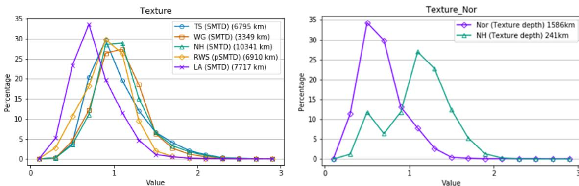
**Figure 6-1 Whole network results for the local authority comparison for texture depth (left) and comparing Norfolk and NH (right)**
