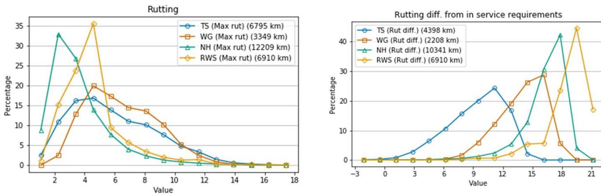
**Figure 4-3 Histogram of rutting values, and differences from in service requirements**
