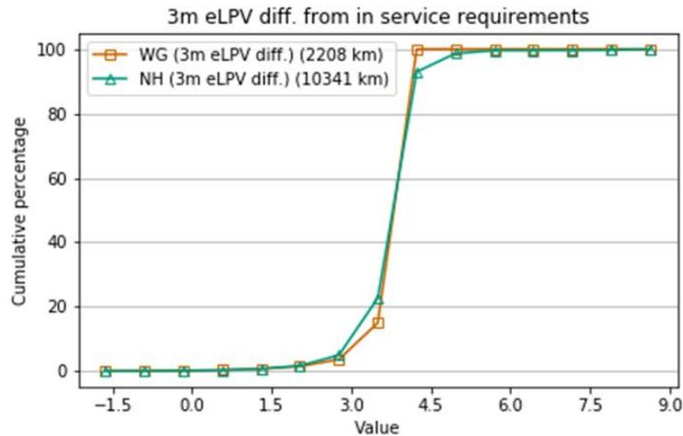
**Figure 3-1 Example cumulative frequency distribution of differences from in-service requirements: 3m eLPV**
