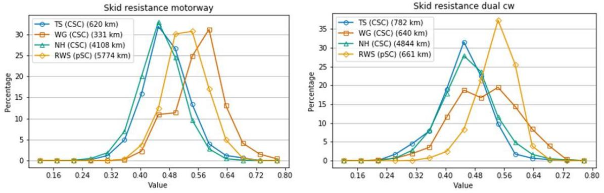
**Figure 4-9 Histograms of skid resistance values for motorways (left) and dual carriageways (right)**
