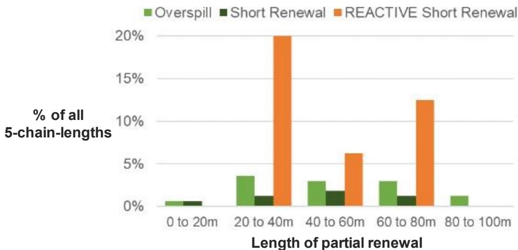
Figure 6 – Histogram of renewal lengths less than the full 5-chain-lengths
