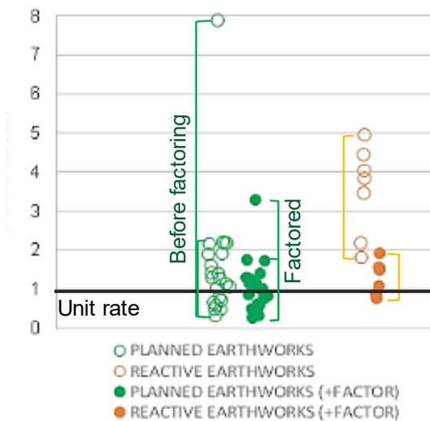
Figure 12 – Hollow dots show costs per effective volume (as shown in Figure 2a); solid dots show the same data, if the unit rates were factored for the items in the simple balance model
