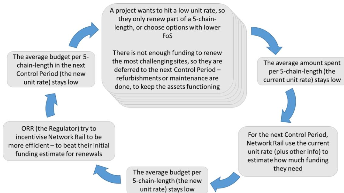
Figure 5 – Flow chart showing how decisions to try and hit low unit rates, lead to unit rates staying low in future Control Periods
