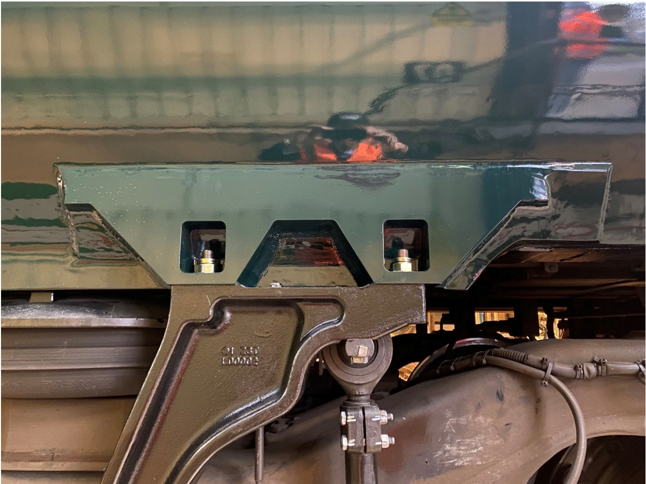
Figure 4.1 Hitachi's modification of bolster area (intermediate vehicle)
