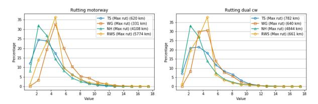
Figure 4-4 Histograms of rutting values for motorways (left) and dual carriageways (right)
