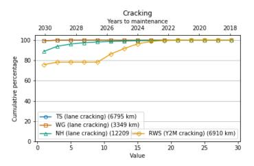
Figure 4-5 Cumulative frequency distribution for cracking values
