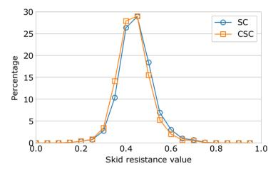
Figure B-1 The distributions of SC and CSC values for a sub-set of the NH network
