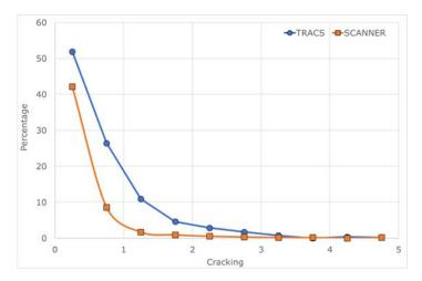
Figure B-2 Comparison of the cracking intensities reported by TRACS and SCANNER on a selected test site
