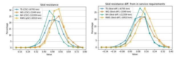
Figure 4-8 Histogram of skid resistance values and difference from in-service requirements
