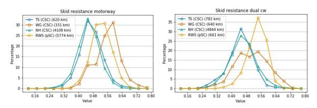
Figure 4-9 Histograms of skid resistance values for motorways (left) and dual carriageways (right)
