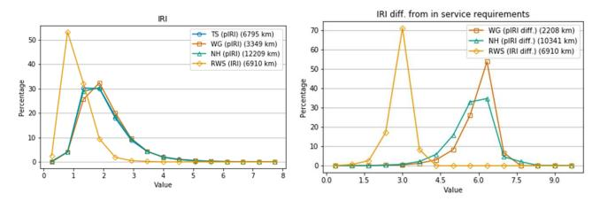
Figure 4-2 Histogram of IRI values, and difference from in-service requirements9
