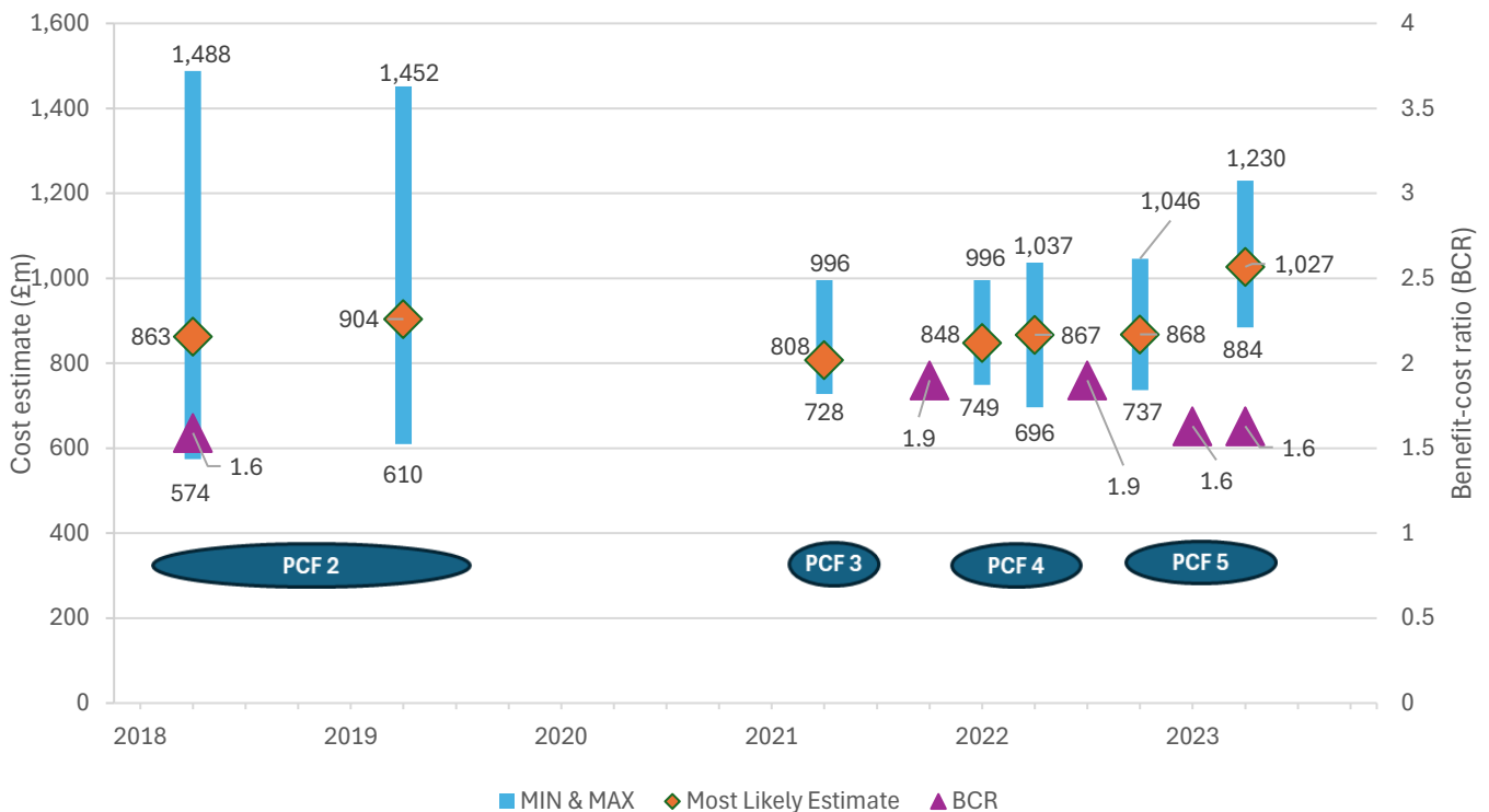
Figure 5.2: Evolution of the A428 cost estimate and BCR through the PCF stages, including portfolio risk (£m, nominal prices)
