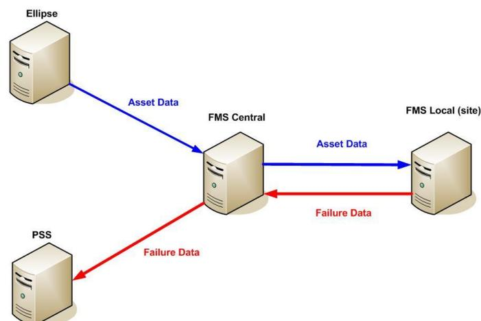
**Figure 14 FMS Hub and Spoke Illustration**
