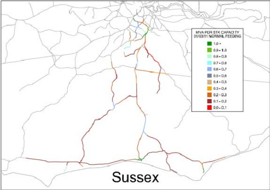
**Diagram 20 Capacity of the Electrification Systems in MVA per STK (Network Rail)**
