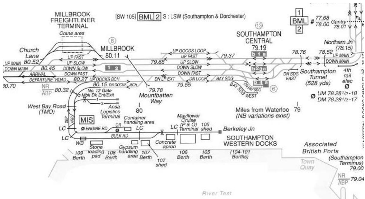
Trains of 520 metres can be accommodated at West Bay Road Crossing without fouling the junction between the Down Docks Branch line and the Up Docks Branch Line at 80 11ch.
