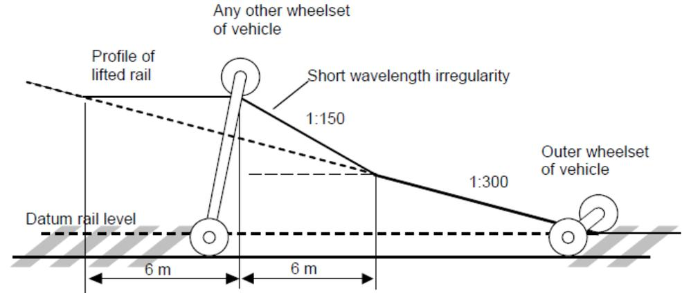
Worst case twist for typical bogie passenger vehicle
