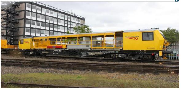
Fitment of a Multi-Purpose Vehicle with a camera array and a track geometry measurement system capable of operating down to 5mph; seeking to extend to ultrasonic testing
