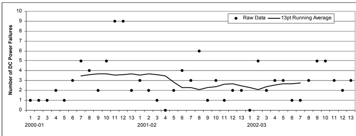
**Figure 5. Trend in the Number of DC Power System Failures.**
