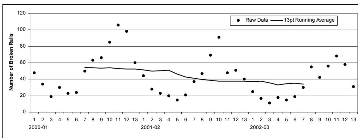
**Figure 1. Trend in the Number of Broken Rails Identified.**
