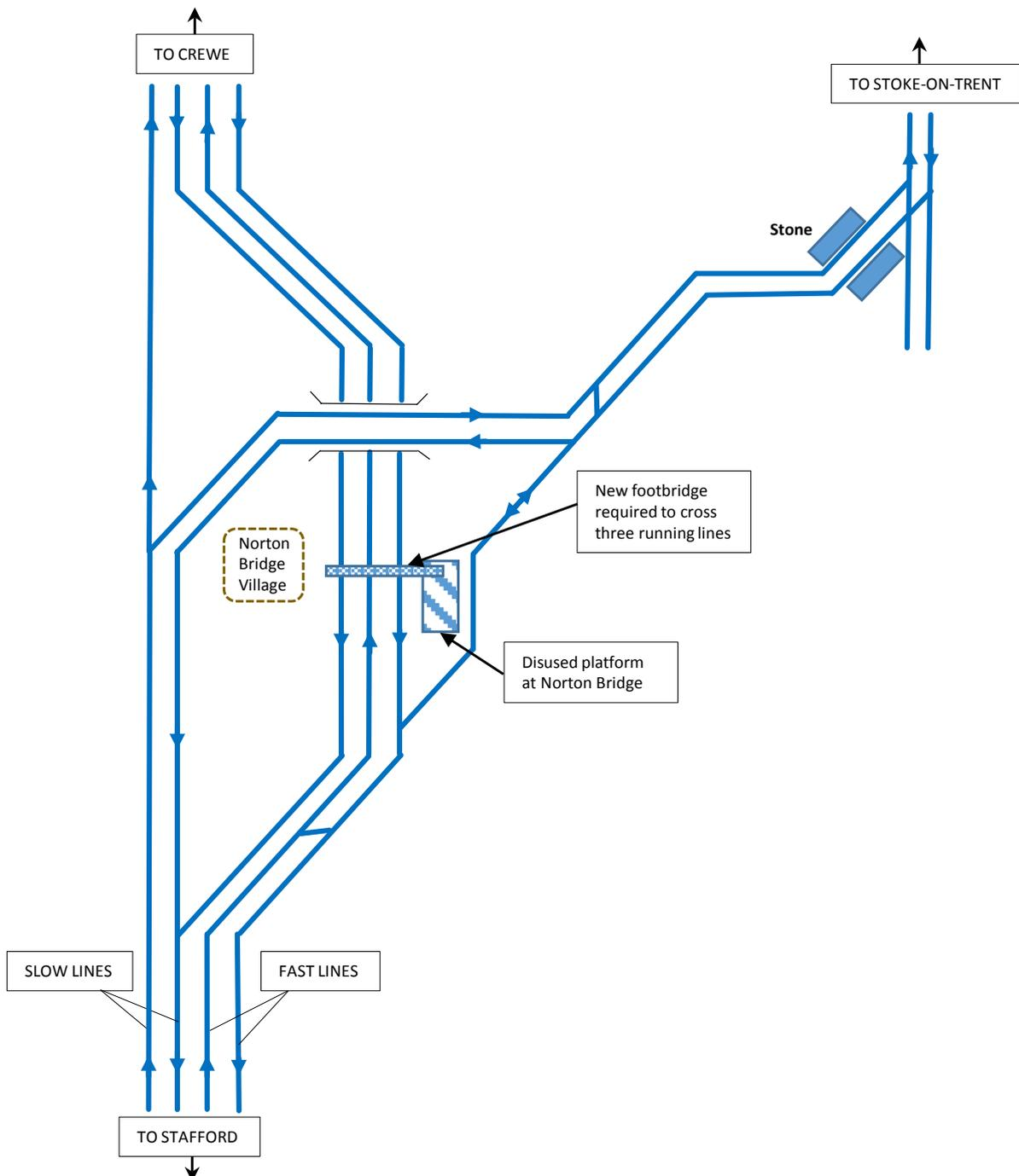
Figure 1 – Diagram showing lines around Norton Bridge
