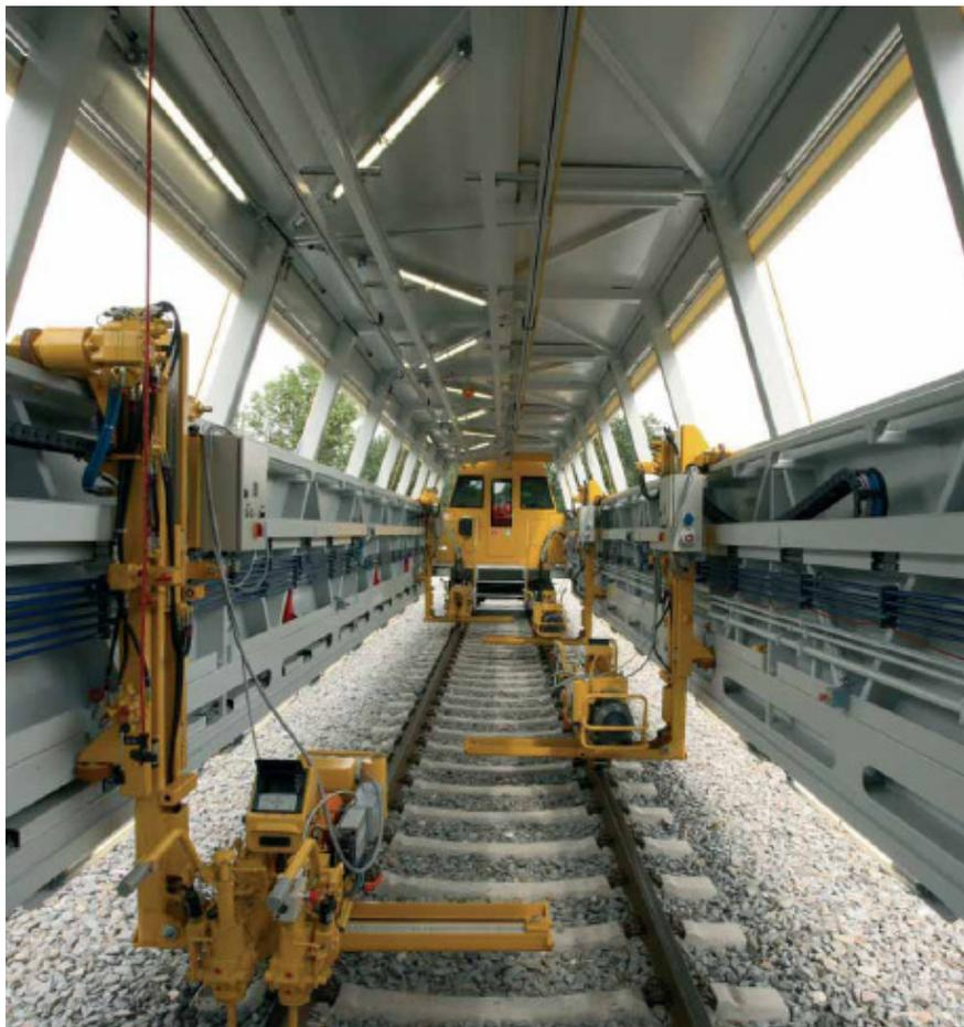
**Enclosed working area of the Robel Mobile Maintenance Unit**
