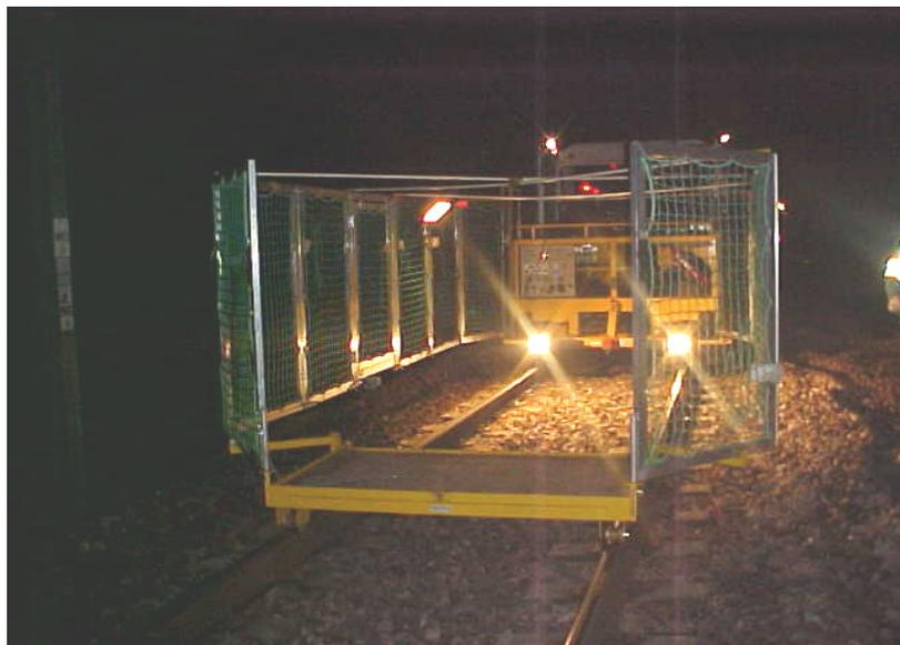
**EDS Barrier system deployed on track**
