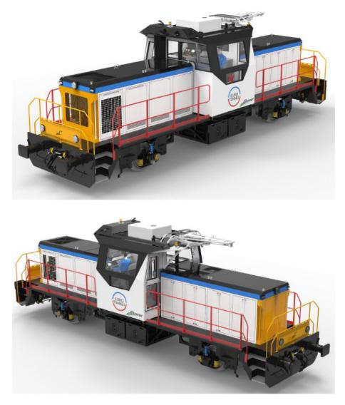
Note: Pantograph is for earthing purposes only during maintenance works.
