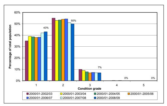
Figure 7.12.2 Average condition grade of a.c traction contact systems (M15)
