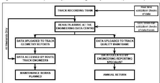
Figure 7.3.5 Process map of compilation and reporting of track geometry data
