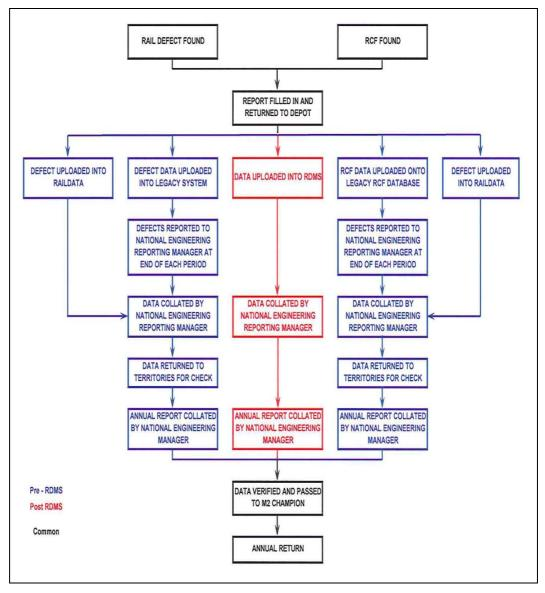
Figure 7.2.3 Process map of rail defects recorded in RDMS
