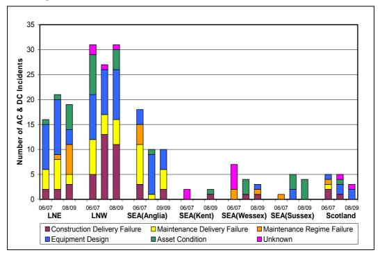
Figure 7.9.3 Comparison of a.c. and d.c. Incidents by Failure Analysis Category (M11 & M12)
