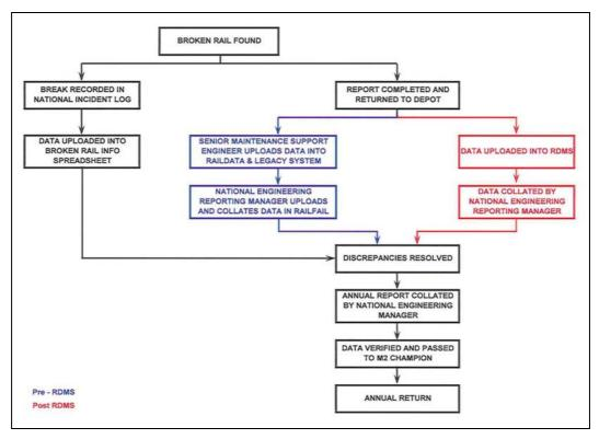
Figure 7.1.3 Process map of broken rail recording in RDMS
