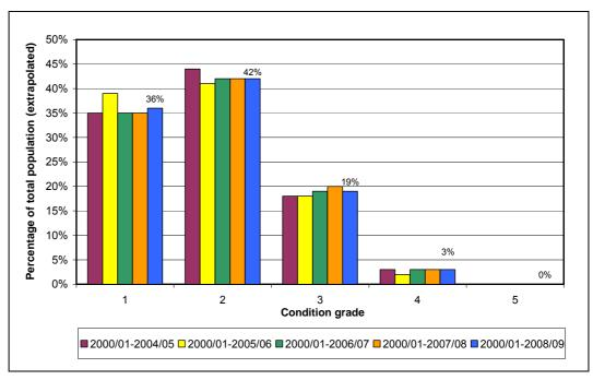
Figure 7.13.2 Average condition of conductor rails (M16)
