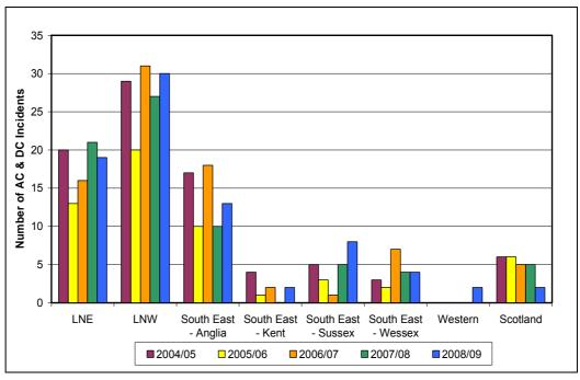
Figure 7.9.2 Number of a.c. and d.c. Incidents causing over 500 minutes delay (M11 & M12)
