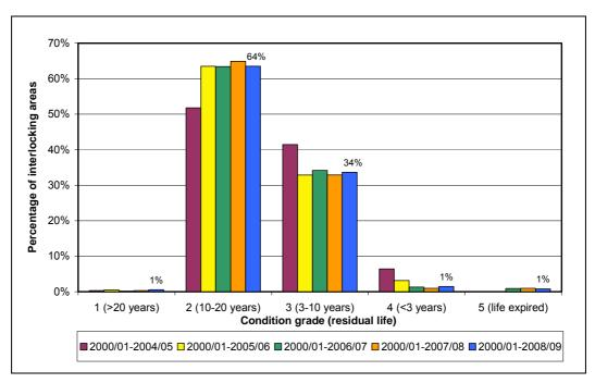
Figure 7.8.1 Average signalling asset condition (M10)
