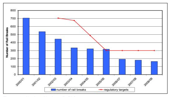
Figure 7.1.1 Number of broken rails (M1)
