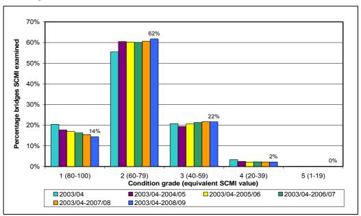
Figure 7.6.2 Bridge condition reported during the last six years (M8)
