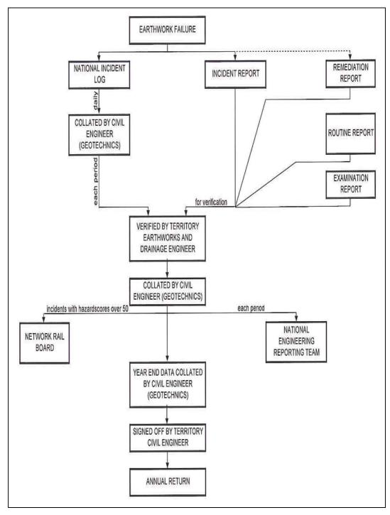
Figure 7.5.4 Process map of data acquisition, verification and reporting of M6
